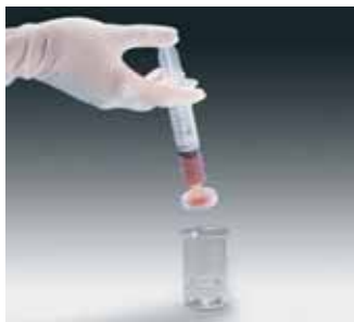
Sartobind MAs may be used by hand or with a chromatographic system via Luer Lock adapters.
